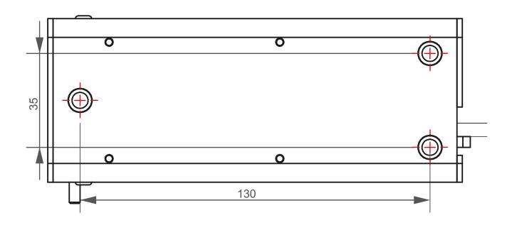
Please note: 3x M6 screws are required Recommended screw length inside unit: 10mm
