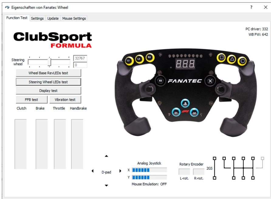
Indicator bar shows the current steering wheel position, the upper box shows the position in digits, the lower box shows the position as an angle (positive and negative angle related to the calibrated wheel center position).
