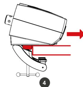
Tighten the table clamp (B) by turning the table clamp screw (C). Ensure that the table clamp's feet remain well aligned with the bottom of the table plate.
