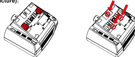
**IMPORTANT:** Use only good quality M6 bolts. Choose the correct bolt length to prevent the thread from reaching more than 16 mm into the wheel base. **Example: If your table is 20 mm thick, the bolts must not exceed a total thread length of 36 mm!** Always use all three hard-mount points as this allows for a proper and stable installation and avoids damage!
