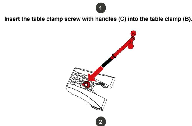
Turn the table clamp screw (C) into the bottom center of the CSL Elite Wheel Base (A).
