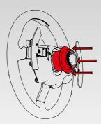
Slide steering wheel off CSL Elite Wheel Base axle.
