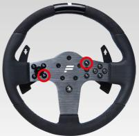
For ClubSport steering wheels press buttons **START (10) + Tuning Menu button** at the same time while H-pattern shifter is connected.
