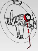
**IMPORTANT:** Tighten only by using the short lever of Allen key!
