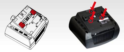
**IMPORTANT:** Use only good quality M6 screws. Choose the screw length so that the thread does not reach more than 16 mm into the wheel base. Example: If your table thickness is 20 mm the screw must not exceed a total thread length of 36 mm! Always use all three hard-mount points, this allows a proper and stable installation and avoids damage!
