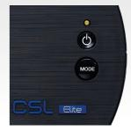
NOTE: Once the mode was changed manually the CSL Elite Racing Wheel will remember the last active mode and will boot in the same mode next time. Exception: After firmware update was done.
