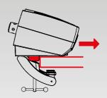
Tighten the table clamp by turning the table clamp bolt. Ensure that the table clamp feet remain well aligned with the underside of the table.
