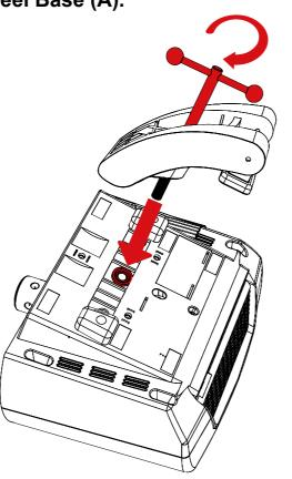
Tighten the table clamp (B) by turning the table clamp screw (C). Ensure that the table clamp's feet remain well aligned with the bottom of the table plate.
