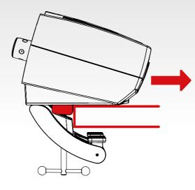
Turn the table clamp screw (C) into the bottom centre of the CSL Elite Wheel Base (A).
