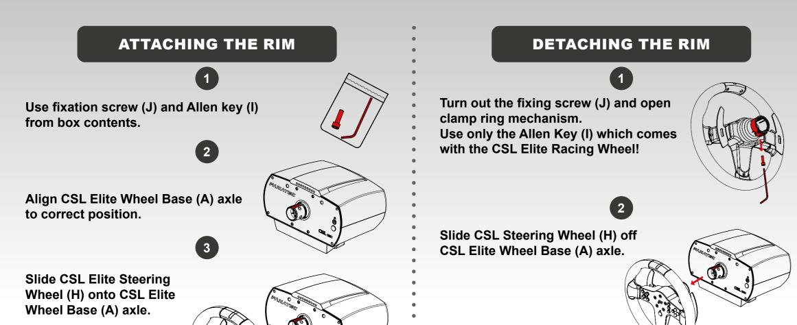
Turn the CSL Elite Steering Wheel (H) top side down to see the bottom side of the clamp ring to follow next step below
