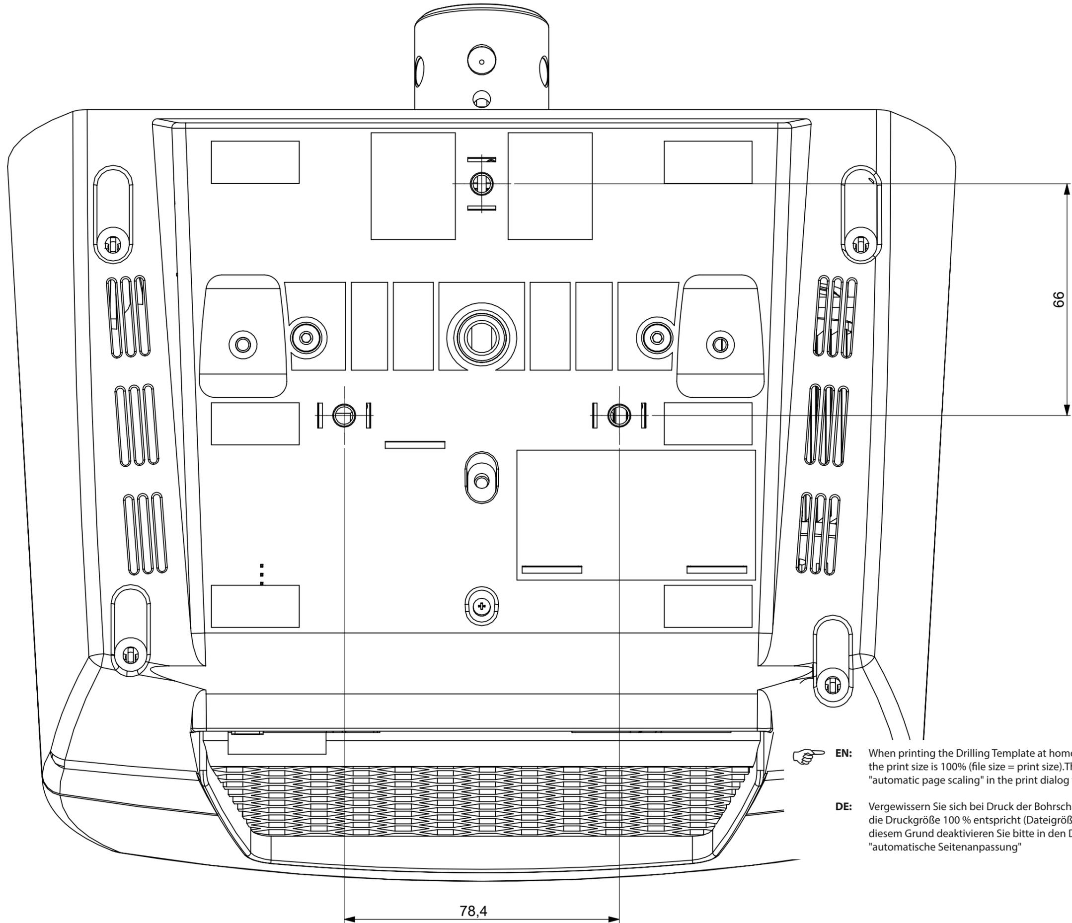
EN: When printing the Drilling Template at home, please make sure that the print size is 100% (file size = print size). Therefore deactivate "automatic page scaling" in the print dialog for example.
