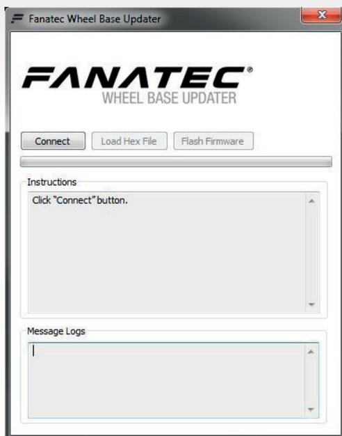
When the Wheel Base Updater is connected to the CSL Elite Wheel Base the buttons 'Load Hex File' and 'Flash Firmware' are available as shown on the right hand side:
