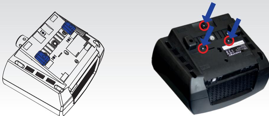
**⚠ IMPORTANT:** Used screws have to be good quality M6 screws. Choose the screw length so that the thread does not reach more than 16 mm into the wheel base. Example: If your table thickness is 20 mm the screw must not exceed a total thread length of 36 mm! Always use all three hardmount points to allow a proper and stable fixation and avoid damages!
