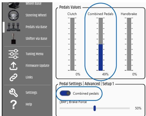
Enabling this option combines the brake and accelerator pedals to operate on a single axis. 49% to 0% is operated by the brake pedal and 50% to 100% is operated by the accelerator pedal.
