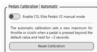
By selecting 'Reset Calibration', the minimum and maximum values of each pedal will be reset to the default values.
