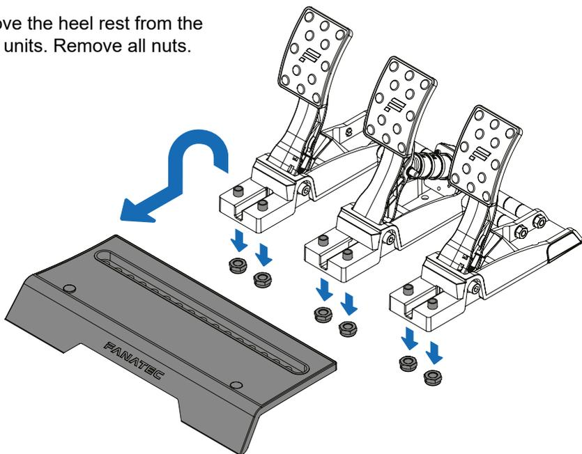
**5** Unscrew all four nuts on the ends of both alignment rods.
