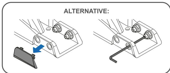
6 Remove the alignment rods and spacers from the pedal units.
