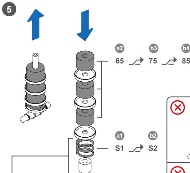
**NOTE:** Always use either the S1 or S2 spring in conjunction with the pre-load elastomer regardless of which configuration you decide on as shown in the box on the right.
