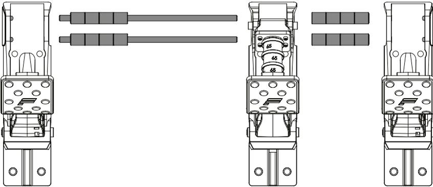
7 Arrange the pedal unit distances or remove as preferred. Examples below:
