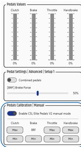
By enabling 'Manual Mode', the minimum and maximum values of each pedal can be manually set throughout the mechanical travel range of each pedal.
