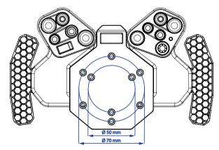
Choose M5 bolts with a maximum thread length of 12 mm. Fanatec Wheel Rims are supplied with the correct bolts. If your wheel rim is not pre-drilled, use the drilling template for the CSL Universal Hub which can be downloaded from the Fanatec website.
