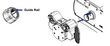
Turn the SQRA clamping nut in the closed lock direction until the indicator line is completely hidden as illustrated below.
