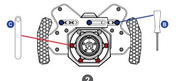
Adjust the horizontal position of modules as desired, then tighten the highlighted bolts and nuts to secure the desired position as illustrated below.
