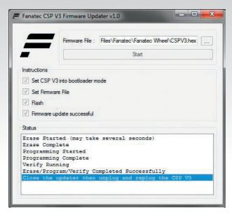
IMPORTANT: The ClubSport Pedals V3 is secured by firmware and by driver so that usually it is not possible to install wrong firmware files on the ClubSport Pedals V3! Do not try to force installation of any wrong firmware to the ClubSport Pedals V3 to avoid damages.
