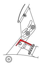
Place the tool to the side of the small grub screw, avoiding interference with the motor cable.
