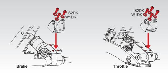
Hang in the damper to the pedal lever at the marked holes and fix it by tightening the two screws S1DK by using Allen Key 4 mm. At brake use the upper holes at pedal arm, at throttle use the lower holes at pedal arm:
