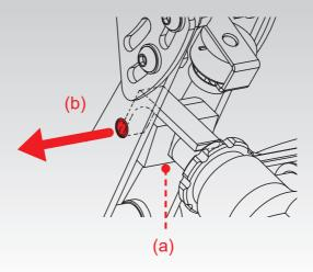
Disconnect the loadcell cable from 'Brake' port at the mainboard and take it out of the cable clips. Then turn the brake assembly downwards out from the brake pedal lever:
