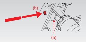
Adjust the preload screw so that the scale is within the correct use range and there is no mechanical play in brake pedal. Note: Preload screw cannot be used in the full range as before, its use is limited only to eliminate the mechanical play:
