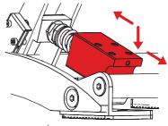
Put the backplate onto the pedalbox again and tighten the two screws with Allen Key 3mm.
