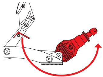
Loosen the small screw (a) with Allen Key 2,5 mm, then remove the thin bolt (b) from the brake pedal lever:
