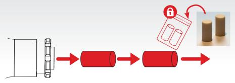
Insert the small Polyurethane spring (E) from Brake Performance Kit package content into the preload screw:
