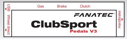
IMPORTANT: Connect the ClubSport Pedals either by USB cable OR by RJ12 cable to a wheel (base). Never connect both ways in parallel to avoid hardware damages!
