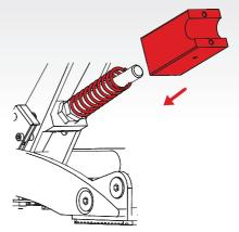
Attach the Pedalbox onto the pedal rod and hang it back into the lower stroke.
