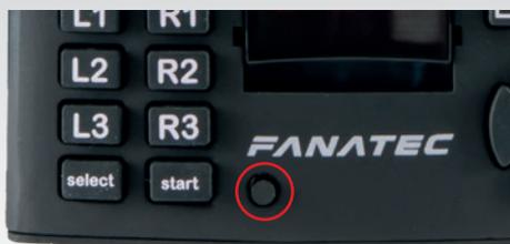
When tuning menu is active then press the buttons **start** + **X** at the same time to calibrate the wheel center.
