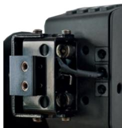
The distance between front side holes and backside holes is 10 mm (center to center). The holes have gears for M5 screws which are also contained in the Universal Hub package.
