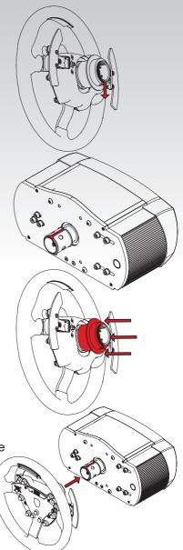
IMPORTANT: Please mind not to use high force to attach the steering wheel to avoid damages! It is possible to attach the steering wheel on the last 8 mm you need a little force because of the O-ring which avoids shaking steering wheels.
