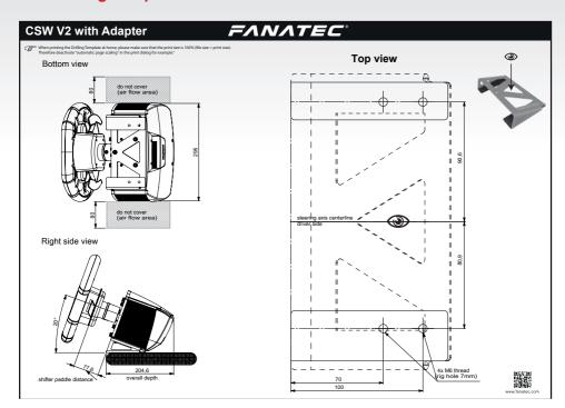
ATTENTION: Please download and print the drilling templates for mounting with and without 20° mounting adapter from the download area of our website www.fanatec.com. Printed drilling templates are included inside the ClubSport Wheel Base V2.5 package.
