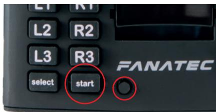
Put the H-pattern shifter's lever into the position shown on the LED display and acknowledge each single position by pressing **START (10)** to get to the next one.
