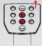
Take off the assembled metal pedal plate and check for the marked holes on throttle pedal arm sides.
