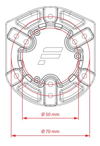
You need to use M5 screws with a max. length of 16 mm in order to avoid a collision with the Podium Hub. The FANATEC® wheel rims come with the correct screws.
