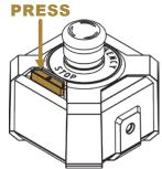
To turn off the wheel base, press and hold the power button for approximately 5 seconds and then release.
