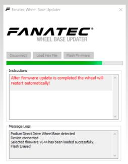
When the update is done the Podium Racing Wheel F1® will restart automatically after firmware update is completely finished (shown right):
