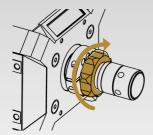
Position the locking ring until it touches the rubber gasket, but do not tighten. This keeps the rubber gasket in place during wheel rim attachment.
