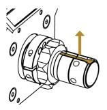
Center the the Podium Wheel Base DD1 PS4™ Quick Release shaft so that the slot is facing up.
