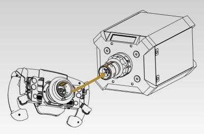
Pull and hold the Quick Release sleeve and carefully push the steering wheel onto the shaft.
