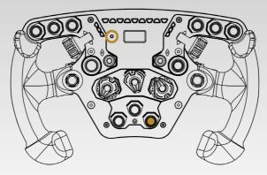
To enter the H-pattern shifter calibration mode press the shown buttons of the ClubSport Steering Wheel F1® PS4™ at the same time while H-pattern shifter is connected, see picture (above).
