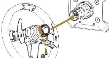
NOTE: When a simplified Quick Release is used, the wheel base automatically limits the torque to prevent damage. ClubSport Quick Releases are required to utilize full torque.
