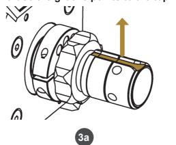
Fanatec ClubSport Quick Release: Pull and hold the Quick Release sleeve and carefully push the steering wheel onto the shaft. Release the sleeve.
