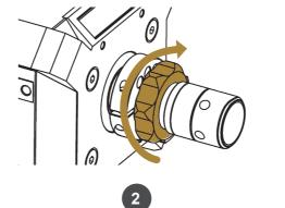
Rotate the shaft so the groove points to the top.
