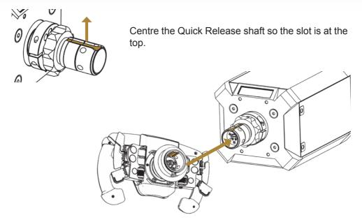
Pull and hold the Quick Release sleeve and carefully push the steering wheel onto the shaft. Release the sleeve.
