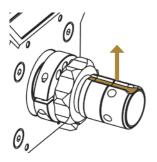
Centre the the Podium Wheel Base DD1 PS4™ Quick Release shaft so that the slot is facing up.
