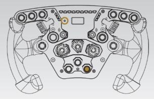
To enter the H-pattern shifter calibration mode press the shown buttons of the ClubSport Steering Wheel F1® PS4™ at the same time while H-pattern shifter is connected, see picture (above).
