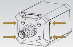
IMPORTANT: Use only good quality M8 bolts. Choose the bolt length so that the thread does not reach more than 20 mm into the wheel base. Always use all four hard-mount points, this allows a proper and stable installation and avoids damage!
