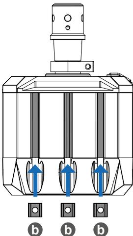
Insert the T-nuts into the T-slots found on the underside of the wheel base for hard-mounting from the bottom.
