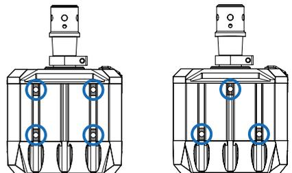
You can position the T-nuts in any configuration to suit the position of the holes on your hard-mounting surface. The examples above show optimal T-nut positions.
