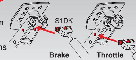
**EN:** Fix damper nut in mounting bracket:
