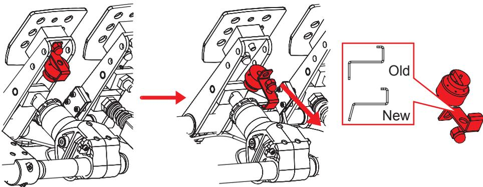
**EN:** Attach the rumble motor upside down with the new rumble motor bracket:
