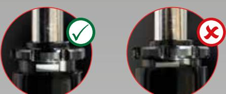
**EN** Minimum preload setting for brake pedal
