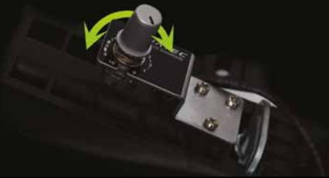
**Brake Sensitivity Adjustment:** You can tune the sensitivity of the brake by making adjustments to the potentiometer. Please note that it is not possible to reach maximum brake pressure when the potentiometer is tuned for the least sensitivity.
