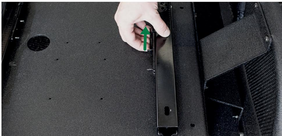
After the assembly of the two screws in the front, adjust the rails forward and mount the two screws in the rear:
