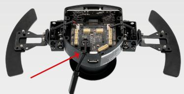
ATTENTION: To use the Podium Button Module Endurance with shifter paddles, they must be attached to the rearward set of mounting holes.
