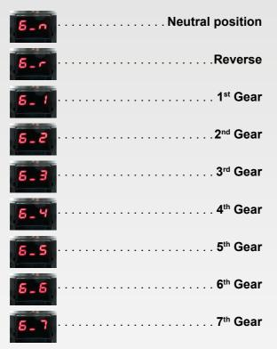
If your shifter has no 7th gear just acknowledge it by pressing  $\langle \blacksquare \rangle$  when the shifter is physically in position of 6th gear. After all gears are calibrated the tuning display shows S\_1 and the shifter is ready for use.
