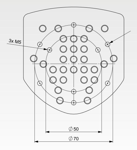
ATTENTION: The maximum torque on the steering wheels bolts must be 3 - 5 Nm, otherwise the thread can be damaged.
