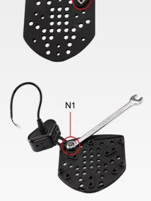
the chosen hole on the frontplate. Turn on a nut N1 (M5 x 7.8 mm x 4.7 mm) onto the bolt thread from the inside of the frontplate. Adjust the lever position according to your favour and to the used rim and then tighten the nut N1 on the bolt S1. The position of the button box or FunkySwitch<sup>TM</sup> is fixed now.
