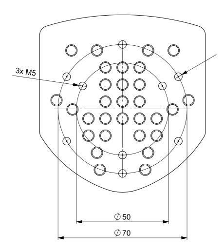
ATTENTION: The maximum torque exerted on the steering wheel bolts must be between 3 and 5 Nm. Over-tightening may result in thread damage.
